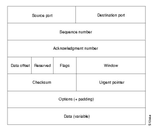
Figure 2 - Transport Control Protocol header [33]
