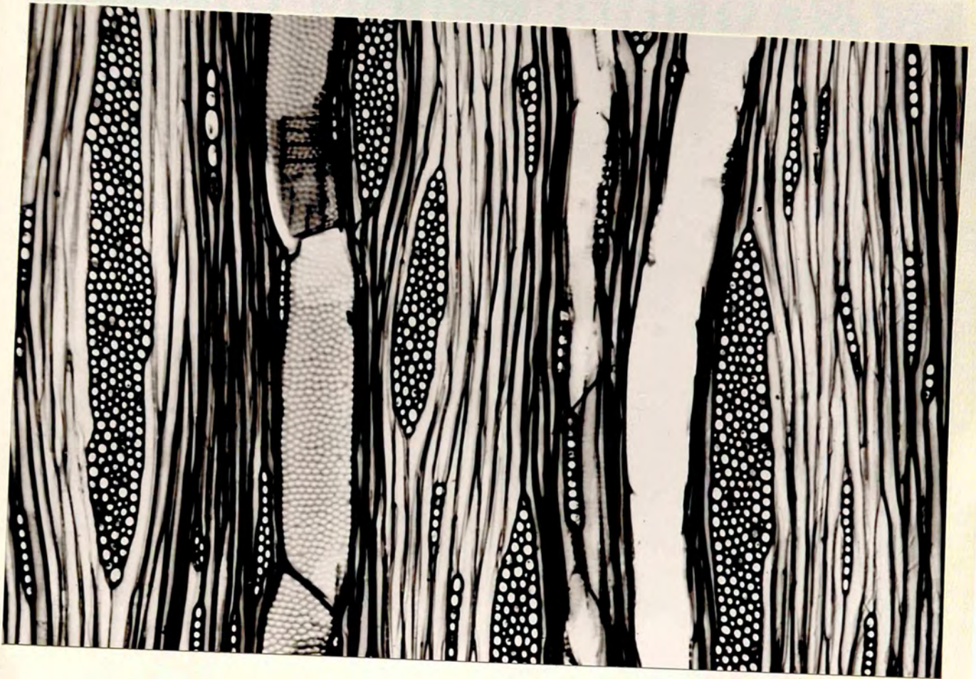
Fig. 31. Acer pseudoplatanus . Photomicrograph of tangential longitudinal section of wood from the bole. x 140
