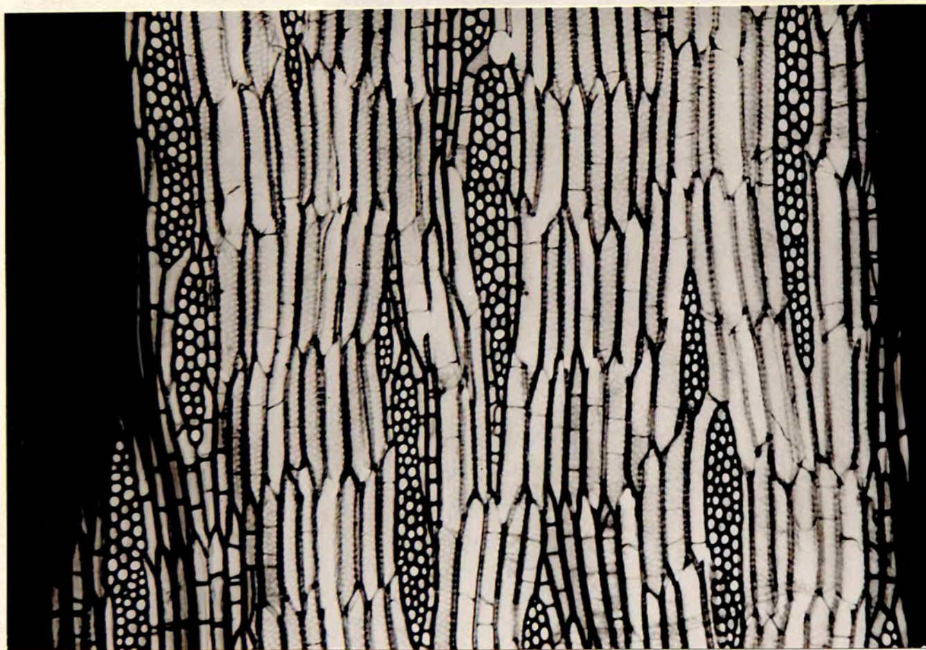
Fig. 32. Robinia pseudoacacia . Photomicrograph of tangential longitudinal section of wood from the bole. x 140.
