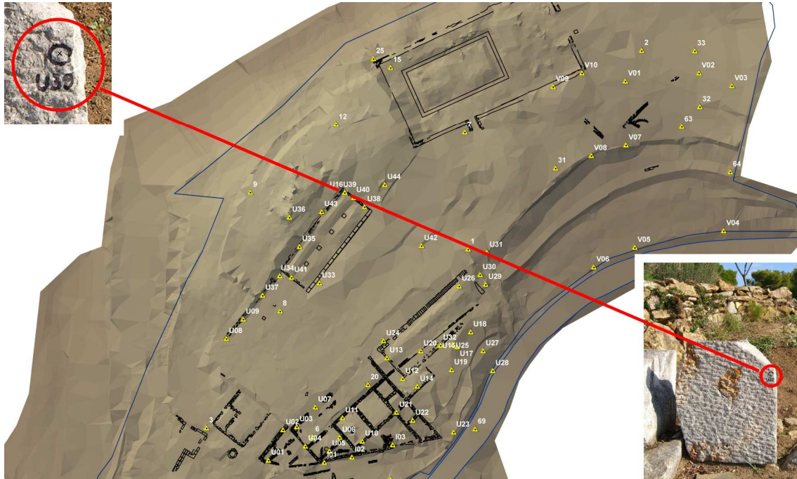
Fig. 5 – Network of fixed points used as backsights for free positioning of the total stations (J. Pakkanen).
