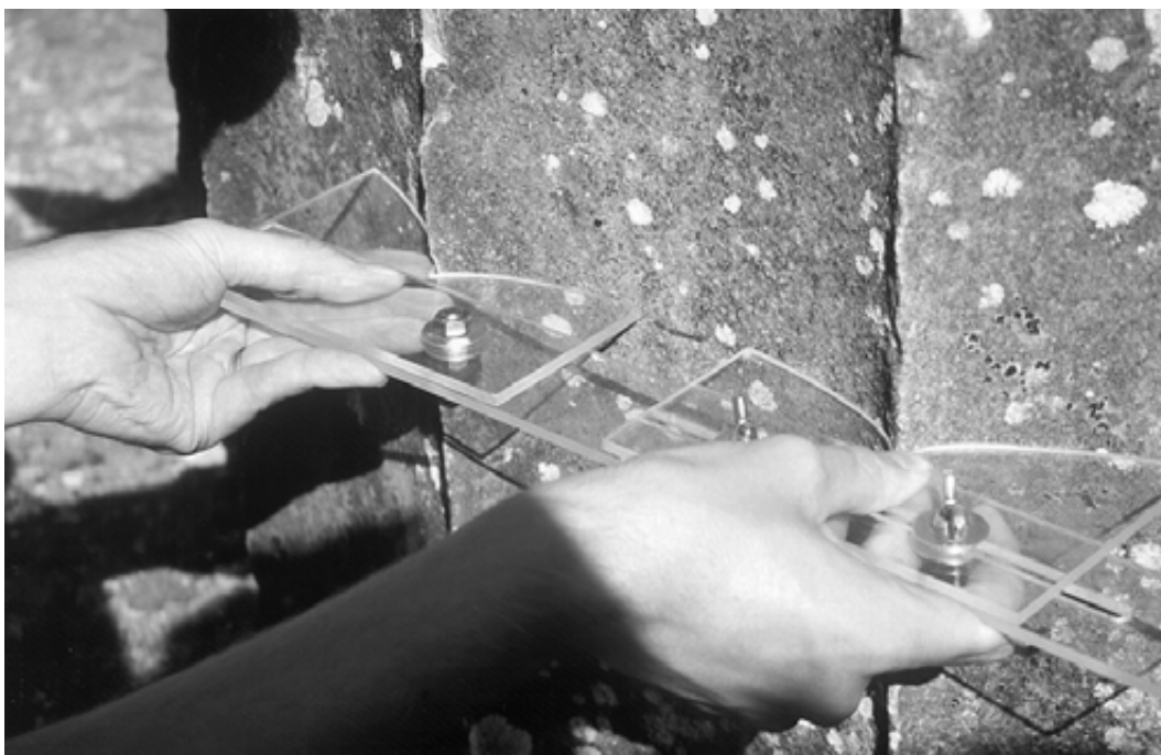
Fig. 7b. Measuring the flute width of block 9 with a special instrument.
