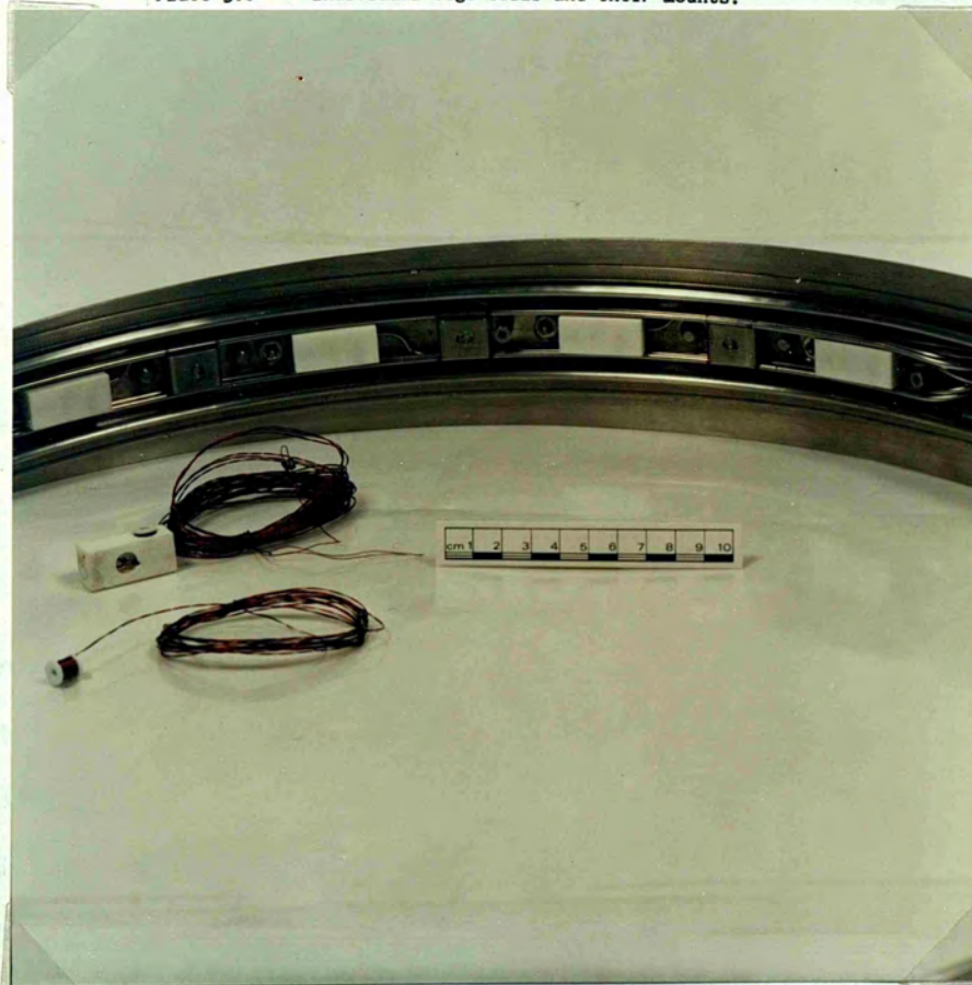
Plate 3.7 Photograph showing a poloidal array of edge coils. The curved metal band into which the coil formers are fixed fits into the inside of the bellows liner.
