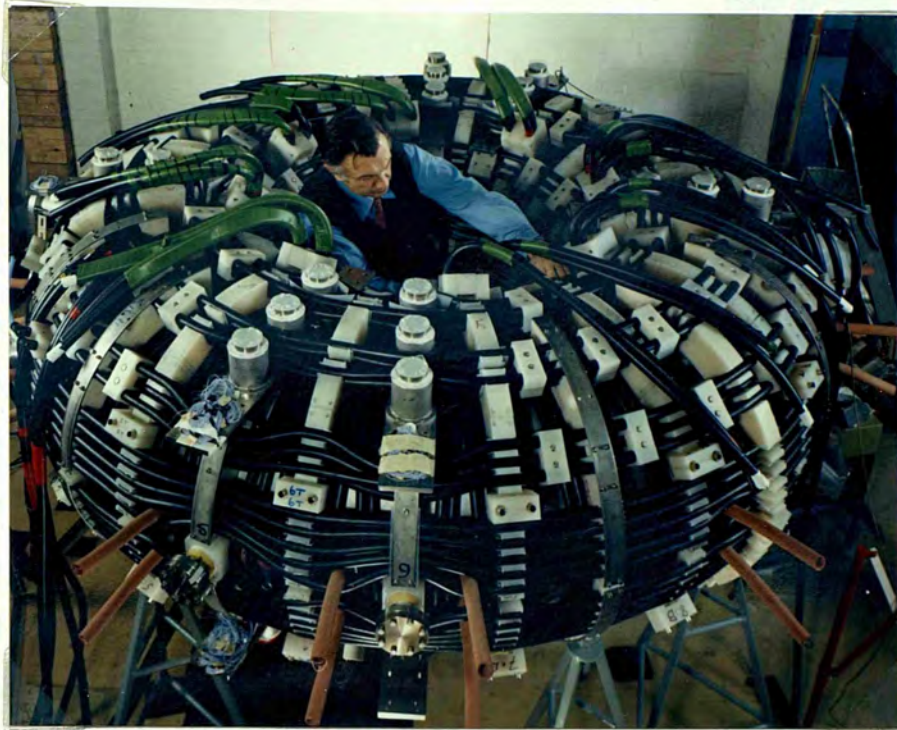
Plate 3.2 The HBTX1A torus before mounting on the iron core.
