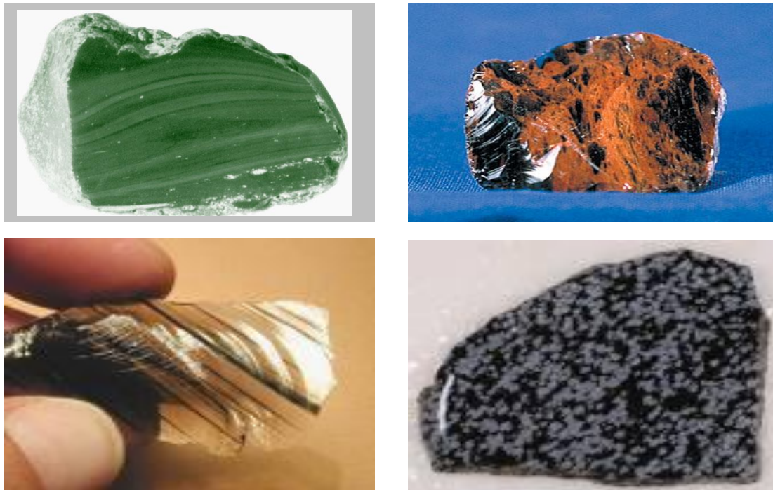
Figure 2.2. Various types of obsidian: green (upper left corner), mahogany (upper right corner), banded (lower left corner) and snowflake (lower right corner).
