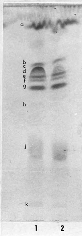
Fig. 15 . One-dimensional two-step TLC separation of complex lipids of mung bean seedlings on silica gel H layer. a, NL; b, CL; c, PA; d, MGDG; e, CMH; f, PG; g, PE; h, DGDG; j, PC; k, LPC. 1 and 2 are both samples. Prewashed solvent: petroleum ether (60°-80°)-acetone (3:1 v/v). Developing solvent: chloroform-methanol-water (65:25:3 v/v).
