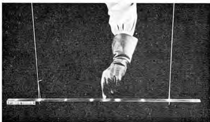
Figure 1. Production of Chladni nodal lines by means of solid carbon dioxide. Frequency, 1317 c./sec.
