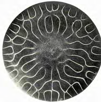
Figures 1, 2. Plate excited at the edge with a bow.
