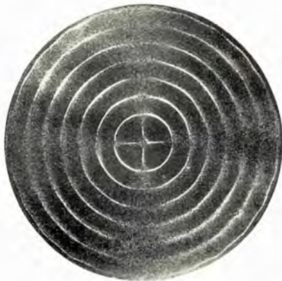
Figures 1, 2. Plate excited at the edge with a bow.
