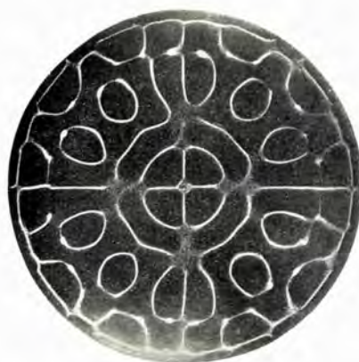
Figures 3 to 6. Plate excited between the centre and the edge with solid carbon dioxide; see table 2.
