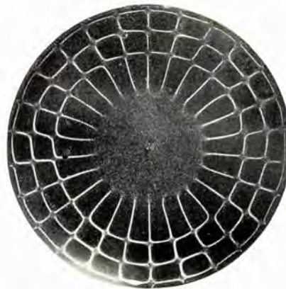
Figures 1, 2. Plate excited at the edge with a bow.
