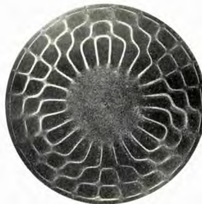
Figures 3 to 6. Plate excited between the centre and the edge with solid carbon dioxide; see table 2.
