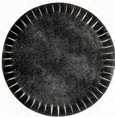
Figures 1, 2. Plate excited at the edge with a bow.
