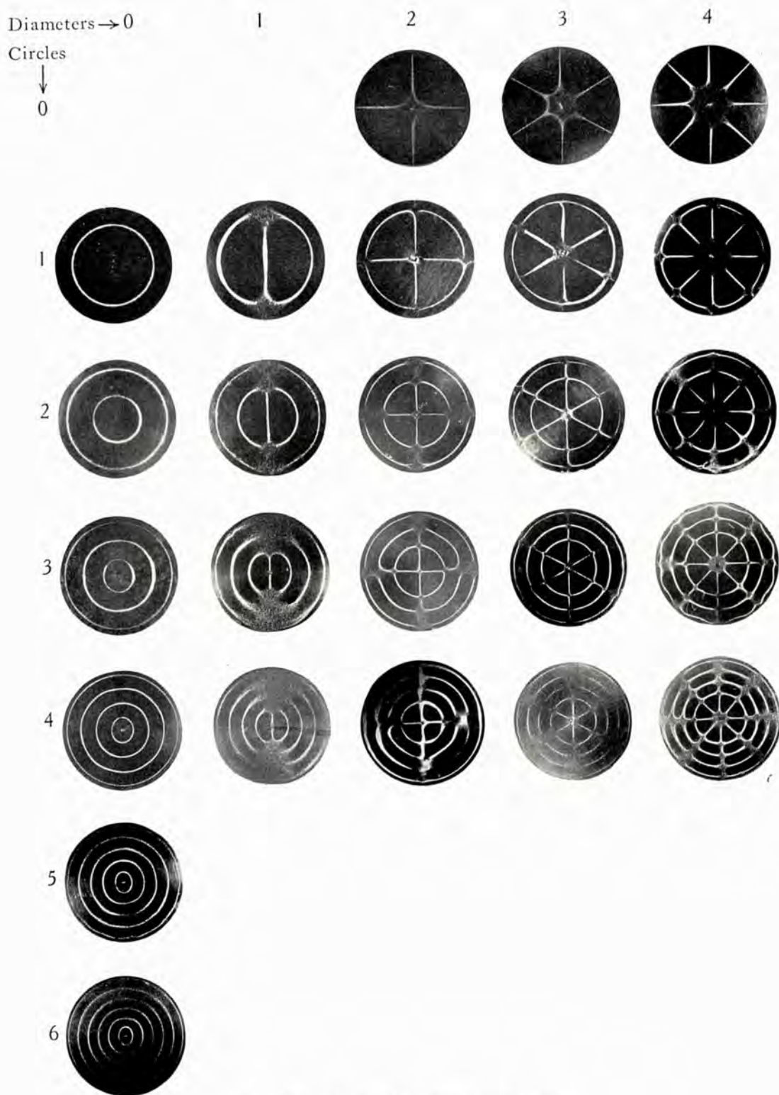
Normal vibrating modes of free circular plate.
