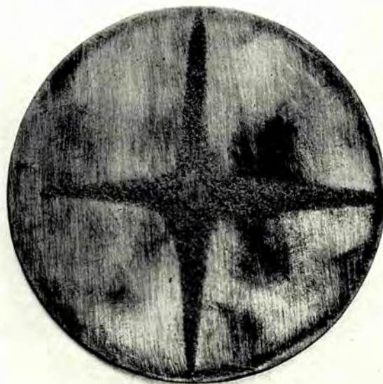
Chladni sand figure on brass disc, produced by contact with solid carbon dioxide. Diameter, 3 in.; thickness, 5 mm.; frequency, 2960 ~.
