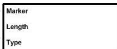
Figure2.6: BGP KEEPALIVE message format
