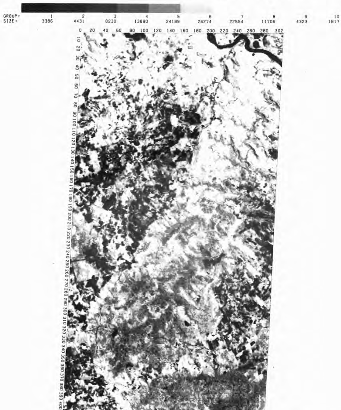
Fig 35. Mangueirinha. Output produced by density slicing and contrast stretching the data in MSS band 7 into ten groups. Output from CCT of Landsat 2. ID 8264112300500. 24 October 1976 overpass.
