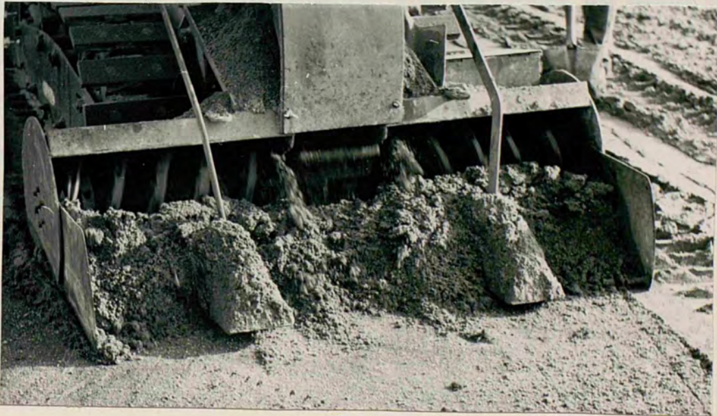
Plate IV. Close up view of skimming mechanism.
