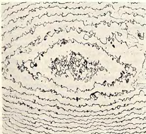
FIG. 1. Multiple beam interference fringes of diamond taken with medium power lens, \times 187.5 .
