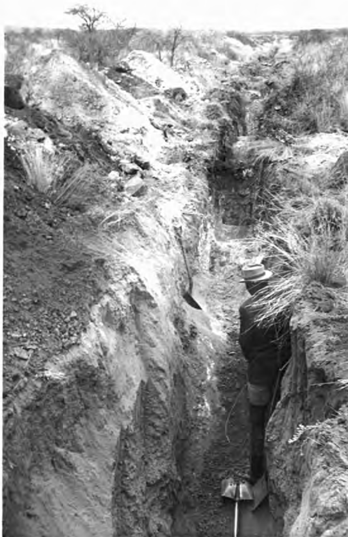
Plate 32 View north-westwards along Trench H.7, northern Okatjirute West. The overburden in this area varies from less than 30cm. to 3m. and consists of calcrete, quartz and quartzite gravel and wind-blown sand. (Ref. MMC/SWA 22/7)
