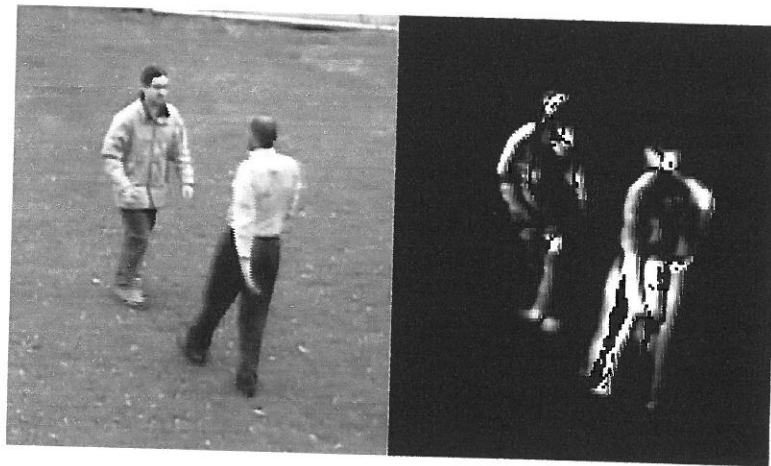
Figure 3.20: Example of contrast free motion detection using non-symmetric filters, as described in Section 3.4.2. The video (left) shows two pedestrians walking towards each other. In the motion image on the right intensity indicates speed only. Edge contrast has been removed and the result is invariant to edge direction. See Figure 3.14 for comparison with DoOG derived motion. Blacked out areas within the pedestrian's motion profile are due to a local lack of edges.
