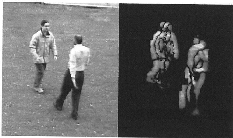
Figure 3.14: Example of DoOG decomposition of video (left) showing two pedestrians walking towards each other. On the right, pixel hue represents motion direction and brightness represents speed. Each pedestrian is represented in a different colour due to their different direction of movement.
