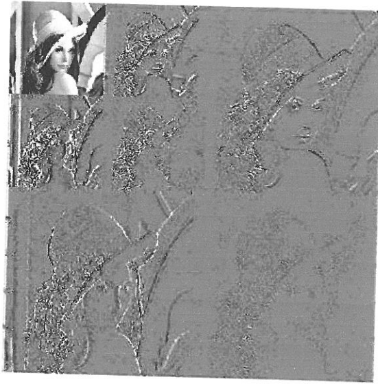
Figure 3.4: Shows the scale pyramid output of wavelet image decomposition. The top row represents the output of the horizontal wavelet, the side column of the vertical wavelet and the diagonal of the diagonal wavelet. The image in the top left column is the result of the final scaling function.
