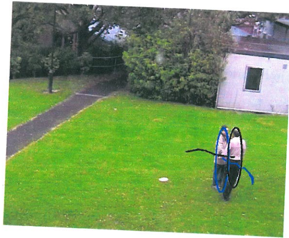
Figure 4.9: Failure of both prediction and appearance model. The pedestrians suddenly stop moving. Their Kalman predicted motion continues and, because they are similarly dressed, the tracks swap onto the opposite targets.
