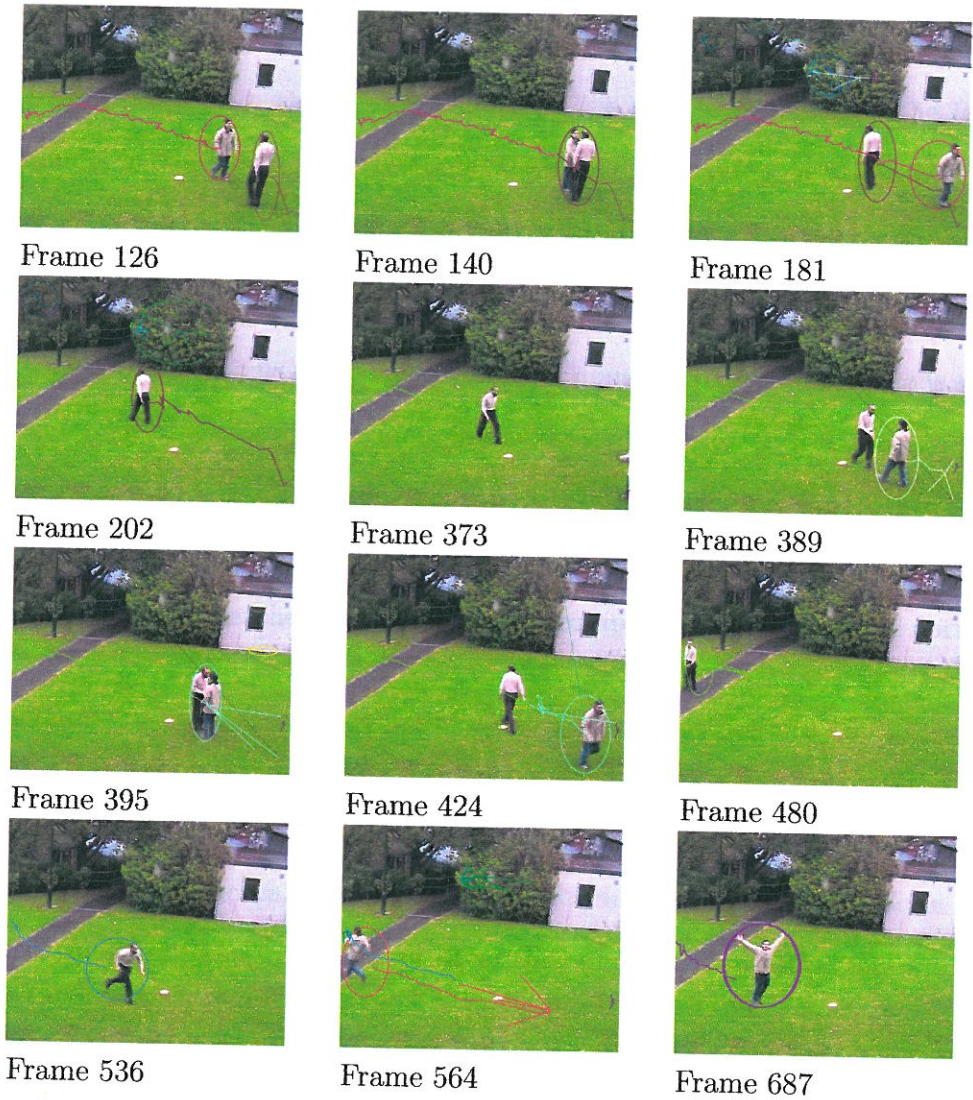
Figure 4.17: Video 3: Video illustrating tracking of dynamically occluding objects. The video also contains a high degree of motion clutter caused by the swaying tree branches and wind. The system successfully tracks the targets despite this.
