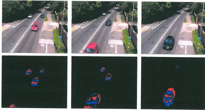
Figure 5.6: Three sample frames from a traffic monitoring video (Top) along with the motion field output (Bottom) produced by the motion distillation stage. Figure 5.7 and Figure 5.8 below contain figures cropped from this data using the object finding and tracking stages.
