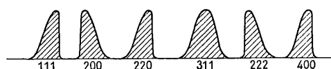
Fig. 6. Effect of combined faulting and segregation on the profiles of powder diffraction lines up to \{400\} .
