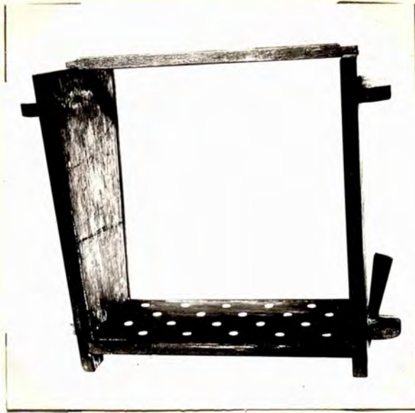
Fig.1. Plant Box for the Observation of Mycorrhiza-formation in situ; the Glass Panels have been removed. \times \frac{1}{4} .
