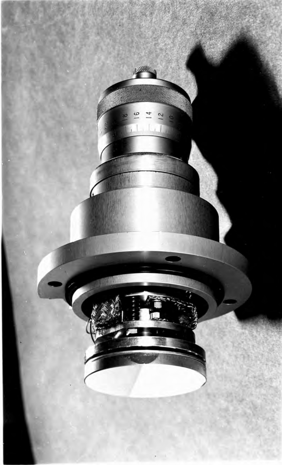
FIG 4.7: THE EARLIER VERSION OF THE PHASE MODULATION SYSTEM - the mirror is attached to the cone of a loudspeaker which is held in an adjustable jig mounted on the micrometer spindle
