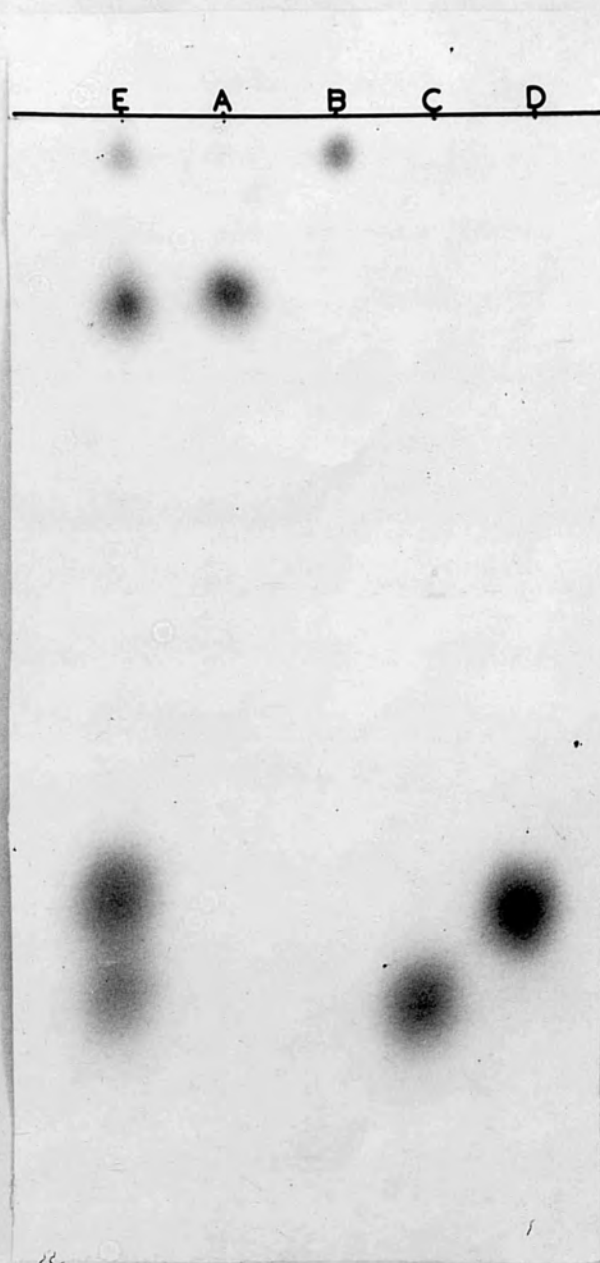
FIG. 30. PAPER CHROMATOGRAPHY OF FERROCENE DERIVATIVES.
