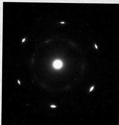
Figure 5.7. Electron diffraction pattern of epitaxial single crystal terbium dihydride films grown on rock salt.
