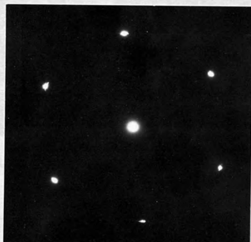
Figure 5.20. Electron diffraction pattern of epitaxial \text{ErH}_2
