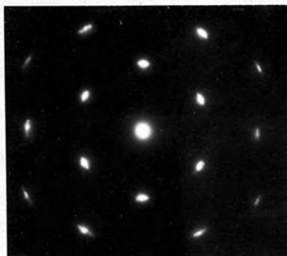
(a) 950\text{A}^\circ (00.1) Tb film grown on (111) rock salt
