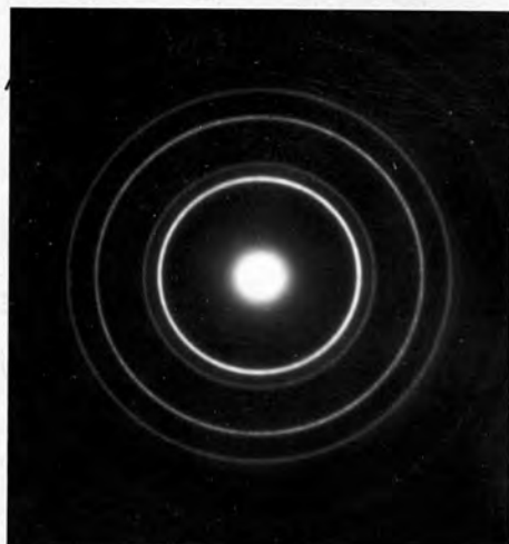
(a) Diffraction pattern of 200Å f.c.c. \text{GdH}_2 before heating in \text{H}_2
