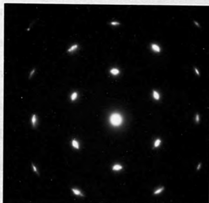
(c) Thickness = 950\text{\AA} , (00.1) h.c.p. Gd grown on (111) rock salt.
