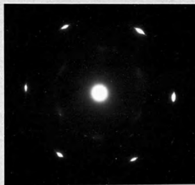
Figure 5.19. Electron diffraction patterns of epitaxial single crystal \text{H}_2\text{O} films.
