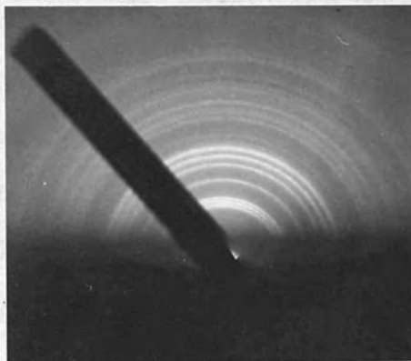
(c) RHEED pattern from the top surface of 1100A film, showing the h.c.p. metallic structure.
