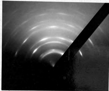
(b) RHEED pattern from the top surface of 650A film, grown epitaxially, showing the co-existence of f.c.c. dihydride and h.c.p. metal.
