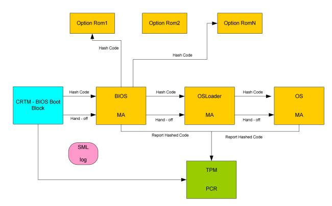
Figure 2: Authenticated Boot Process. Source derived from: Royal Holloway - Trusted Computing Lecture Notes
