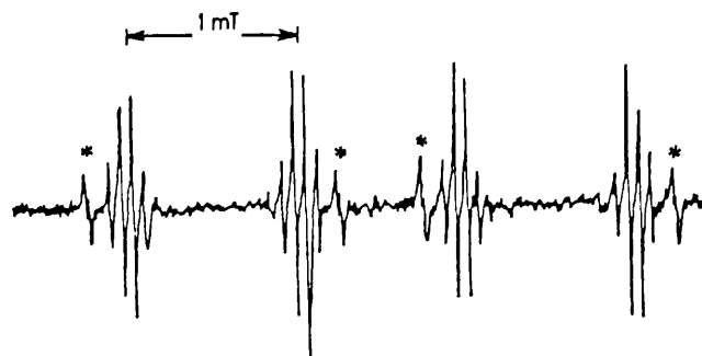
FIG. 1.—E.s.r. spectrum of maleic acid adducts with methyl and hydroxyl (asterisked) radicals.
