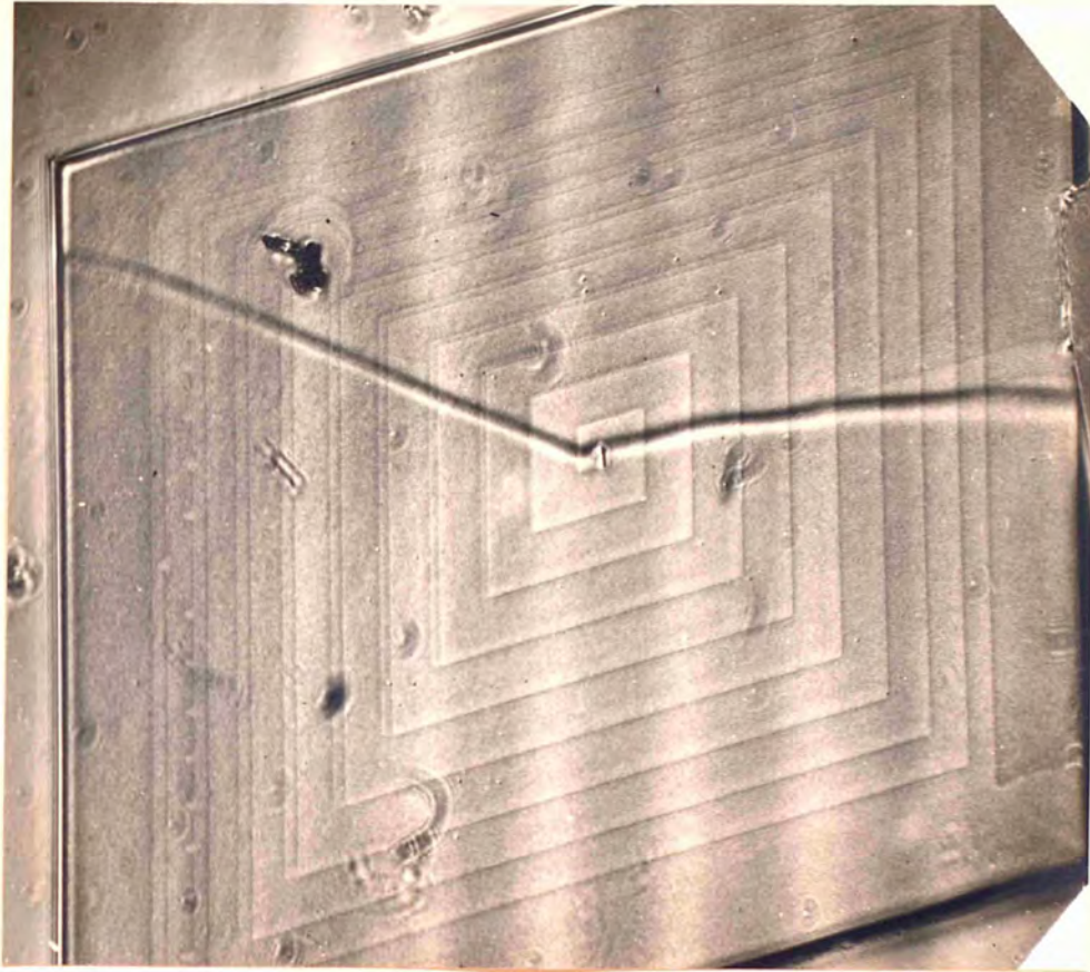
Fig.93. Stearic Acid. Interlaced Spiral. Reflexion Phase Contrast. x530.
