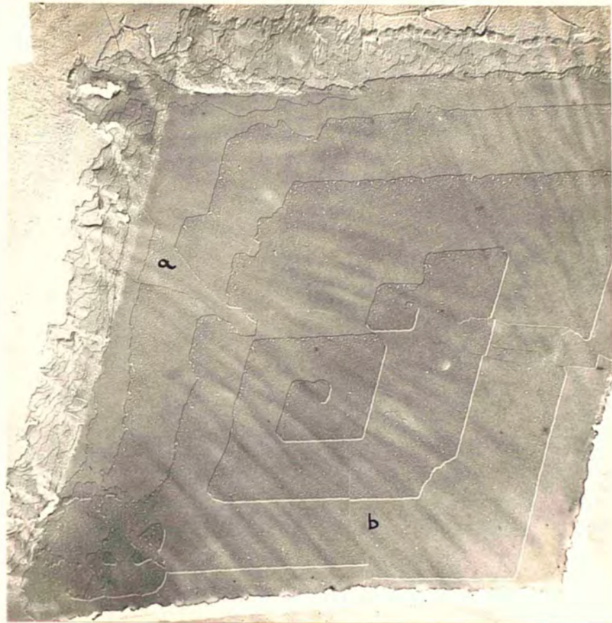
Fig.110. Growth from an Imperfect Dislocation. Electronmicrograph. x9200. Behenic Acid
