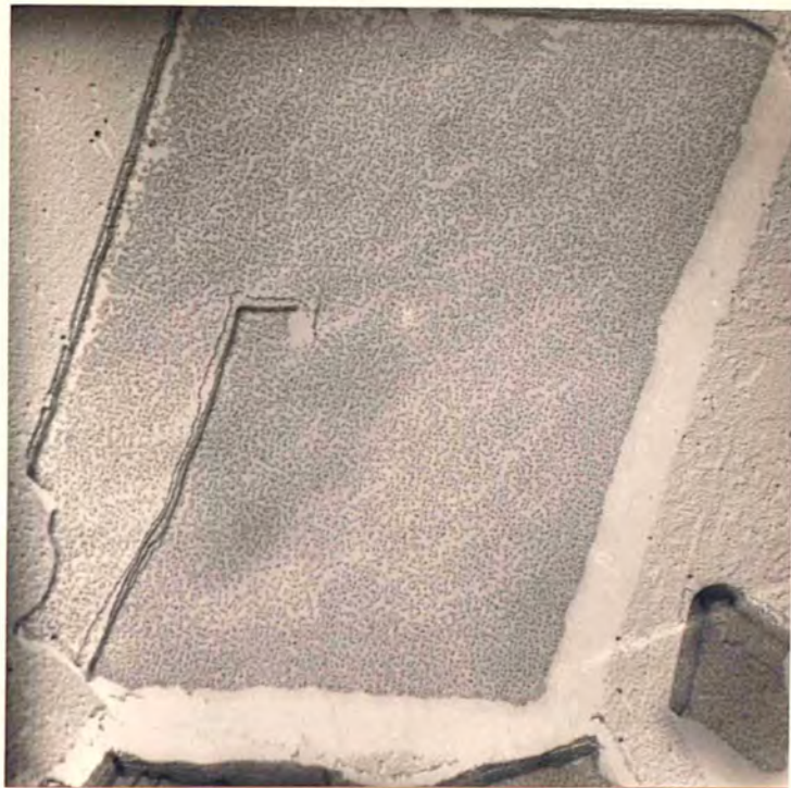
Fig.44. Behenic Acid. Elementary Spiral. Electronmicrograph. x20,500.
