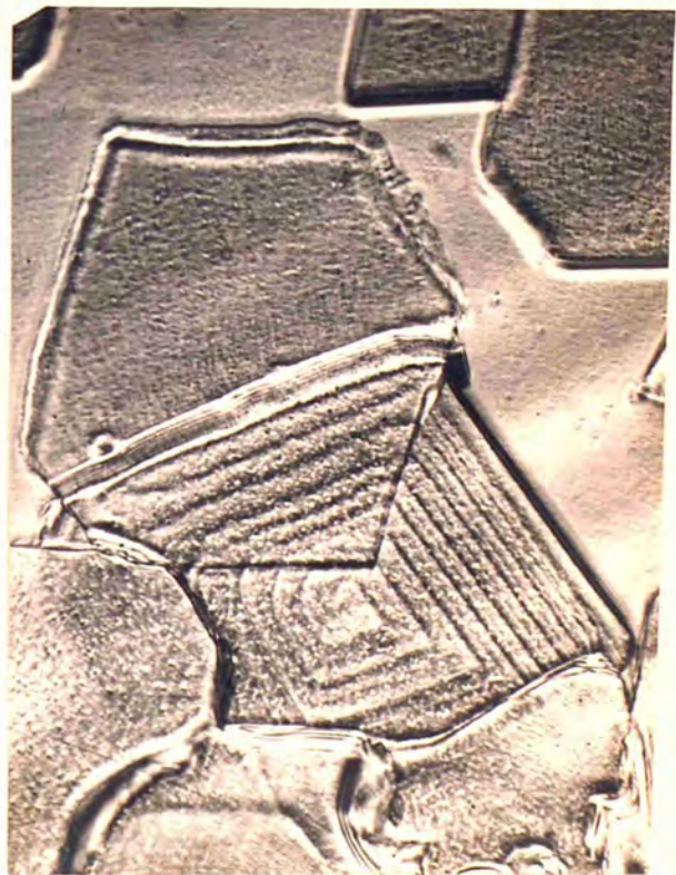
Fig.89. Stearic Acid. Crystal Opaquely Silvered. Reflexion Phase Contrast. x650.
