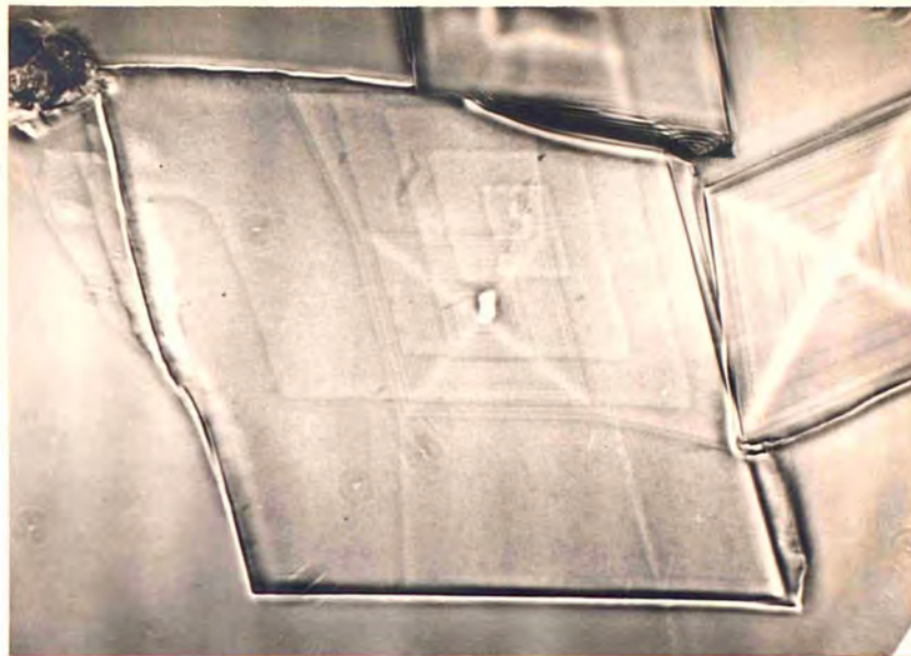
Fig.83. Behenic Acid. Internal Slip, Growth Centres Non-coincident. Reflexion Phase Contrast. x680.
