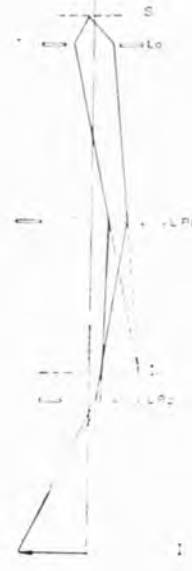
Ray diagram, operation at low magnifications
