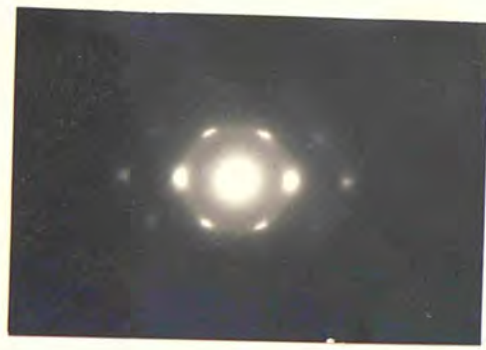
Fig.128. Behenic Acid. Transmission Electron Diffraction Pattern. Incident Beam Normal to Basal Plane.
