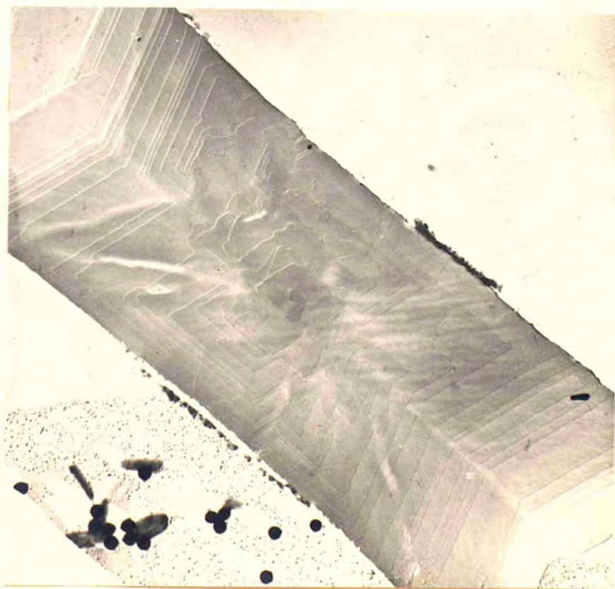
Fig.127. Behenic Acid. Twinned Crystal. Electronmicrograph. x3800.
