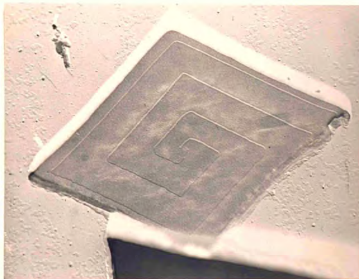
Fig.49. Behenic Acid. Two Spirals of Same Sense, d < 2\pi\rho_c . Electronmicrograph. x5300.
