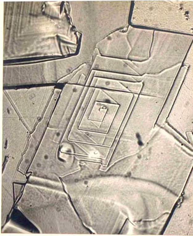
Fig.123. Stearic Acid. Two Spirals in Twinned Orientation. h_2 > d_h > h_1 . \phi = 74^\circ Reflexion Bright-field. x660.
