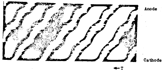
Fig.1. Modulated Argon Discharge, Pressure = 0.46 torr Current = 92 mA, Wavelength = 16.5 cm, Frequency = 2.5 kHz.
