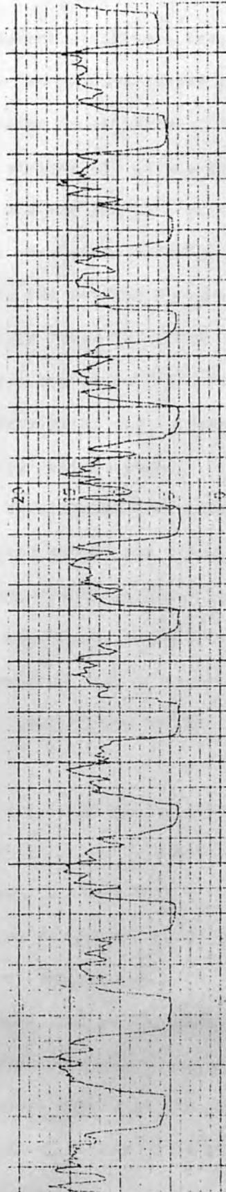
Figure 5.4 Talystep of Grating 4 (Mü1771/2316, 2 1mm -1 , 35m exp.)
