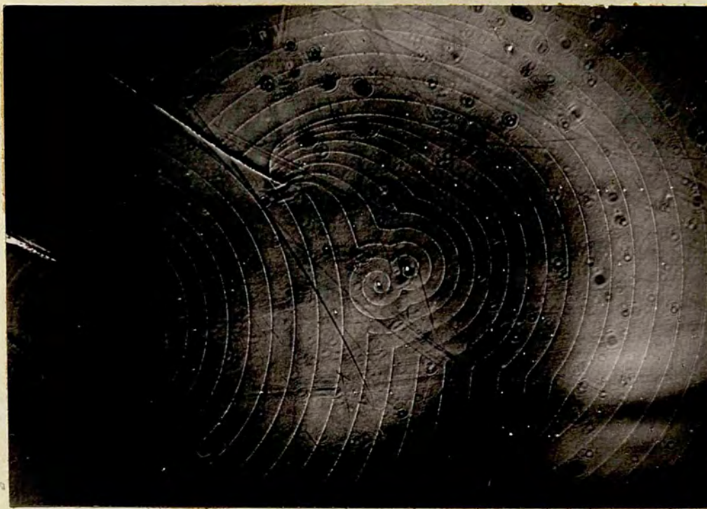
Fig 32. Two left-handed dislocations at a distance > \rho_c .
