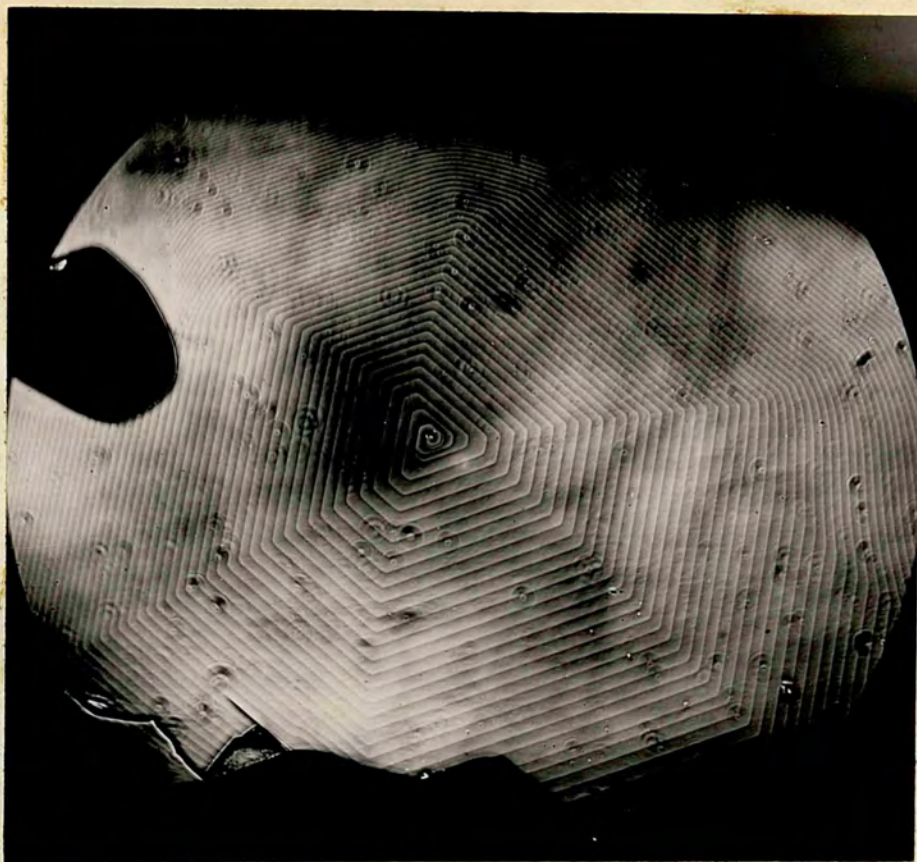
Fig 101. A double spiral observed on Si-C crystal type 33R.
