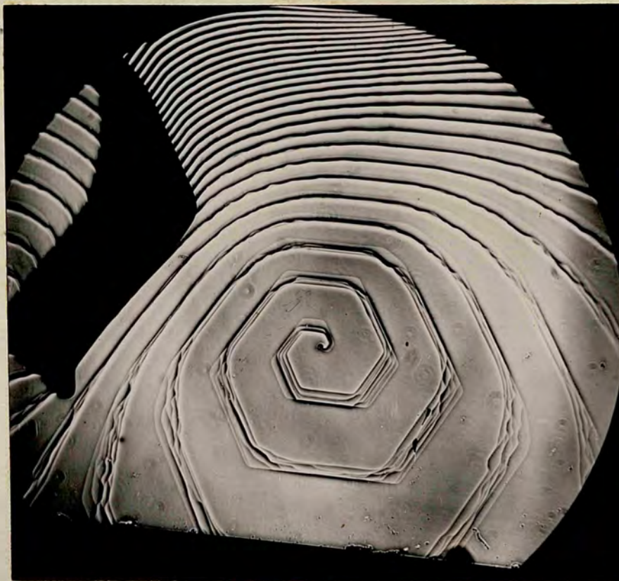
Fig 80. Multiple dislocations with straight edges of growth steps.
