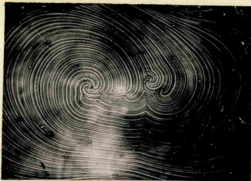
Fig 66. Several groups of dislocations interacting with one another giving rise to a complex pattern.
