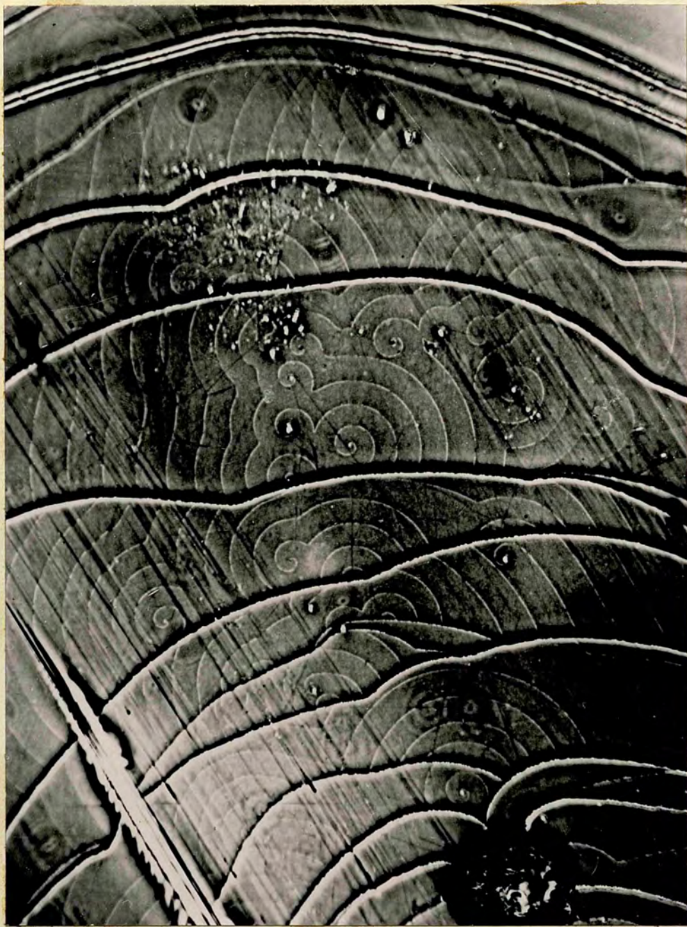
Fig 46. A number of circular growth spirals originating from dislocations of the same sign. Density of dislocation \sim 10^4/\text{cm}^2 .
