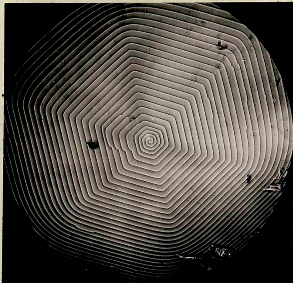
Fig 16b. Hexagonal spiral with step height 130 A.
