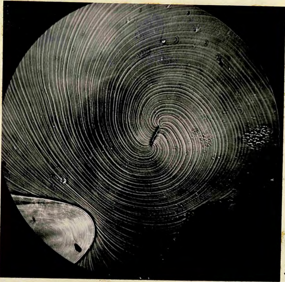
Fig 64. A group of dislocations arranged along a line.
