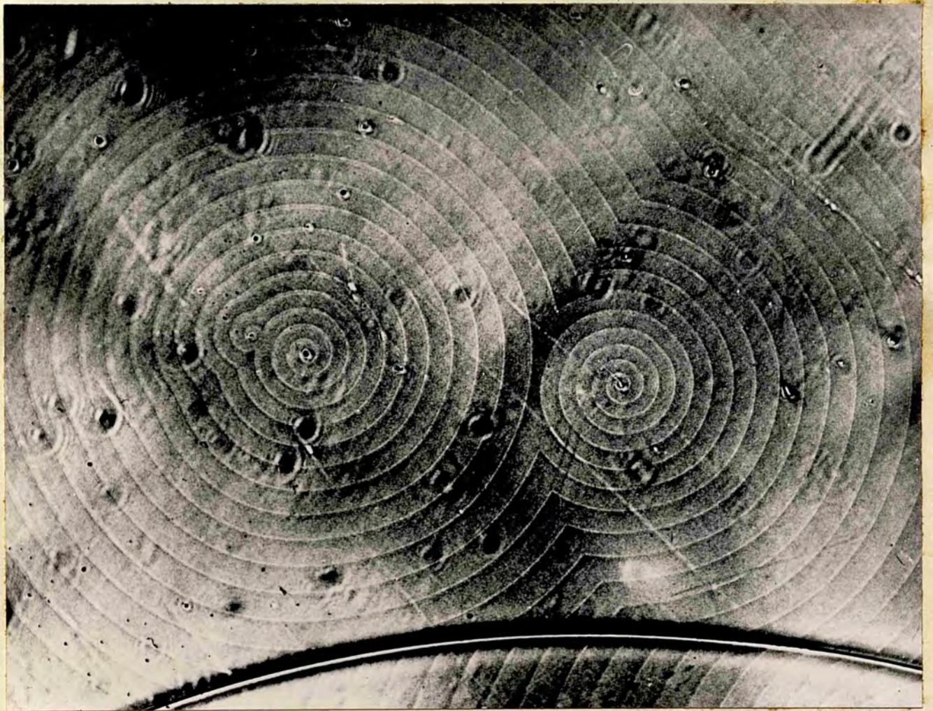
Fig 35. Circular growth spirals; left half illustrating the formation of closed loops (nearly circular) due to two dislocations of opposite sign.
