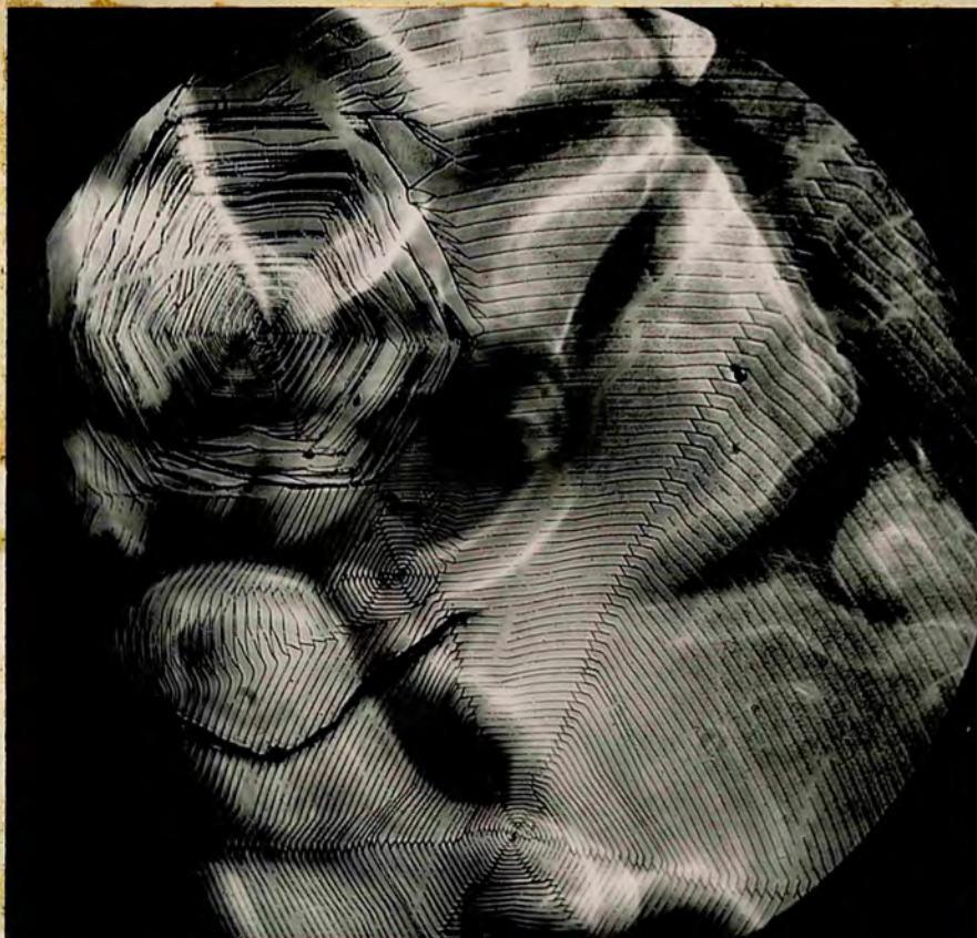
Fig 85. Illustrating several interlaced spirals, (bright field illumination).
