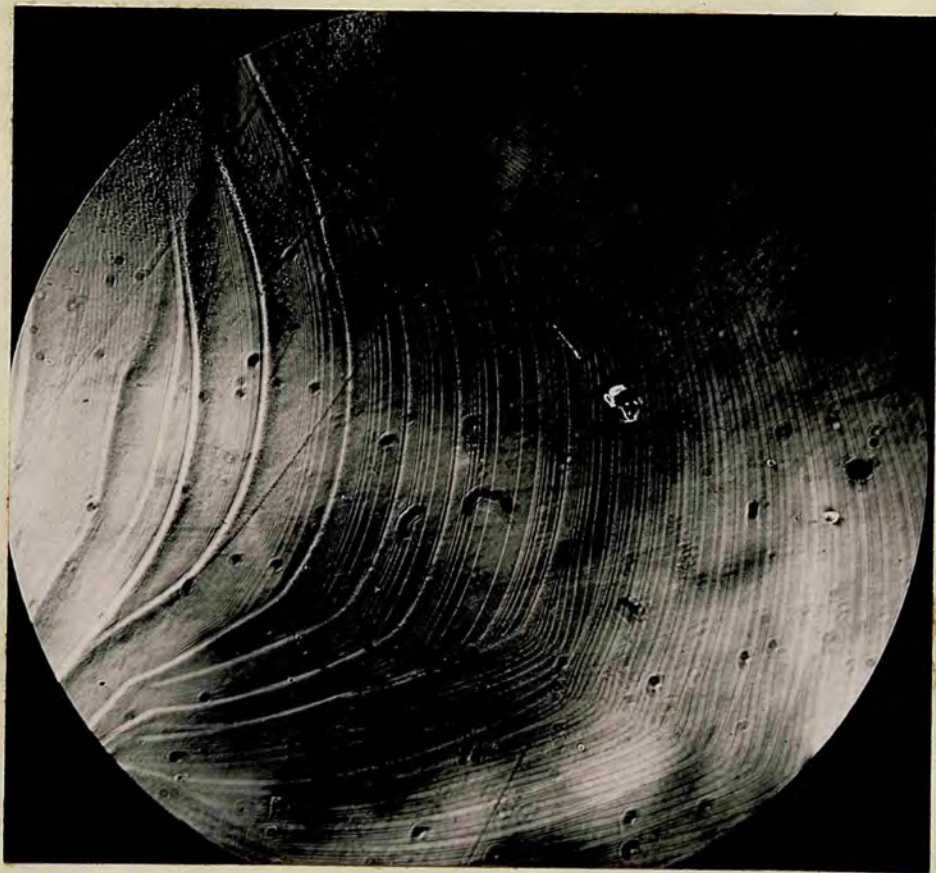
Fig 100. Interlaced spiral with varying number of steps grouping together.
