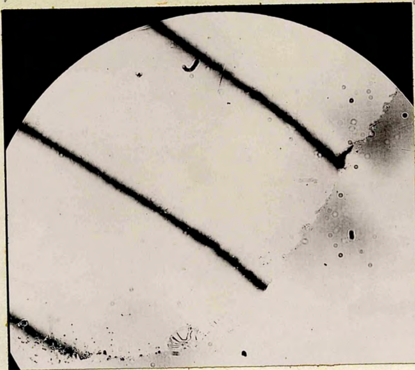
Fig 19b. Fizeau fringes passing over the spiral steps of fig 19a.
