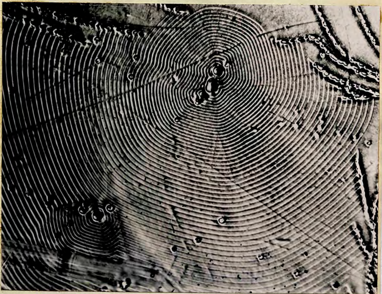
Fig 54. Growth steps terminating at points marked by a series of dots.
