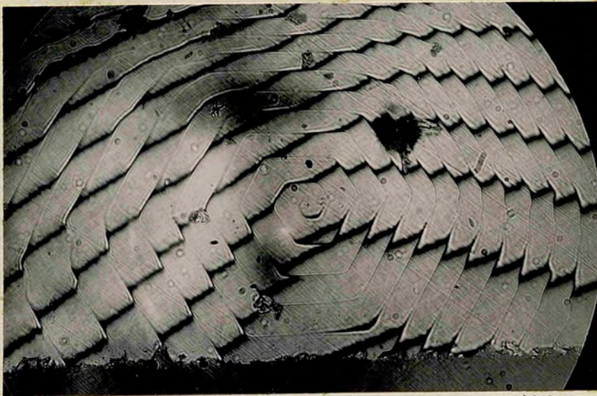
Fig 105. Fizeau fringes passing over fig. 70 by using a lightly silvered glass flat.
