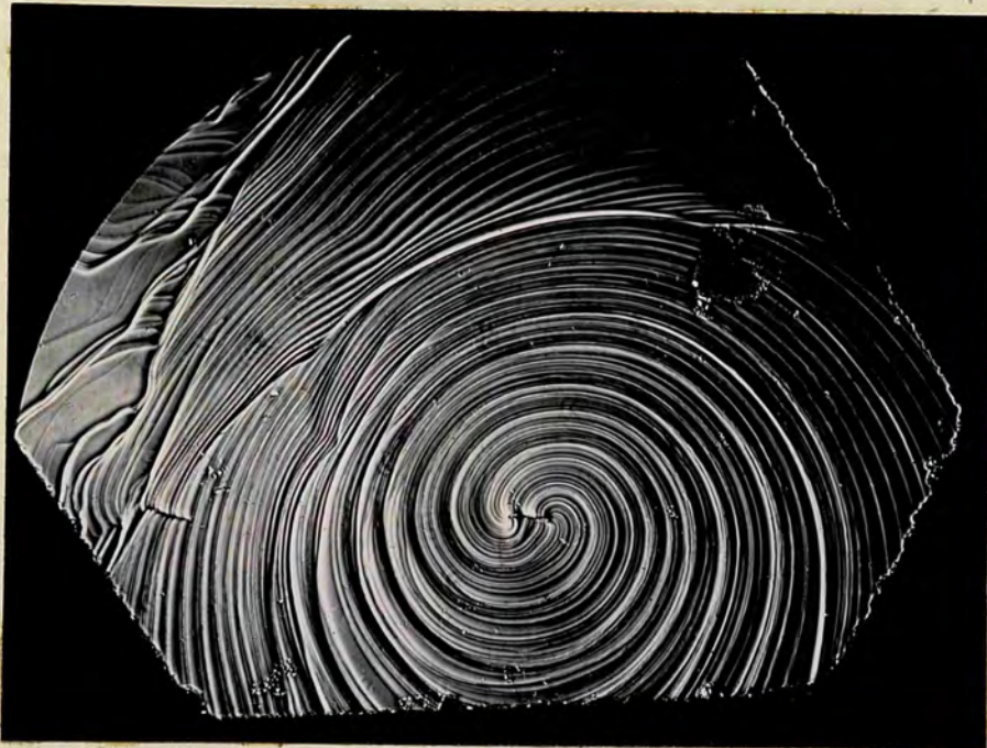
Fig 65. Group of dislocations giving a repeat pattern.
