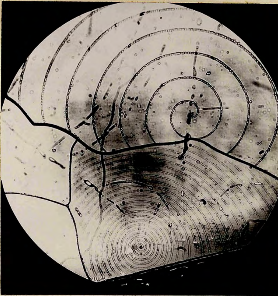
Fig 30. Two screw dislocations of the same sign at a distance < R_c , co-operating with each other.
