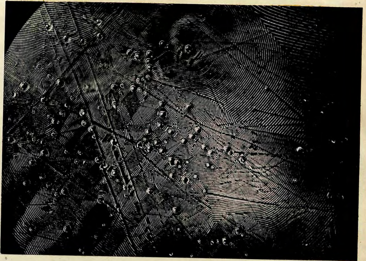
Fig 47. Polygonal spirals originating from dislocations with density \sim 10^5 / \text{cm}^2 , all of the same sign.
