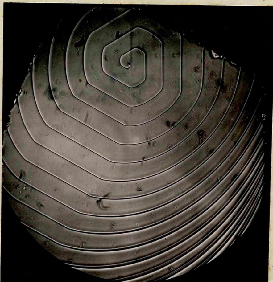
Fig 76. A trigonal spiral with rounded corners.
