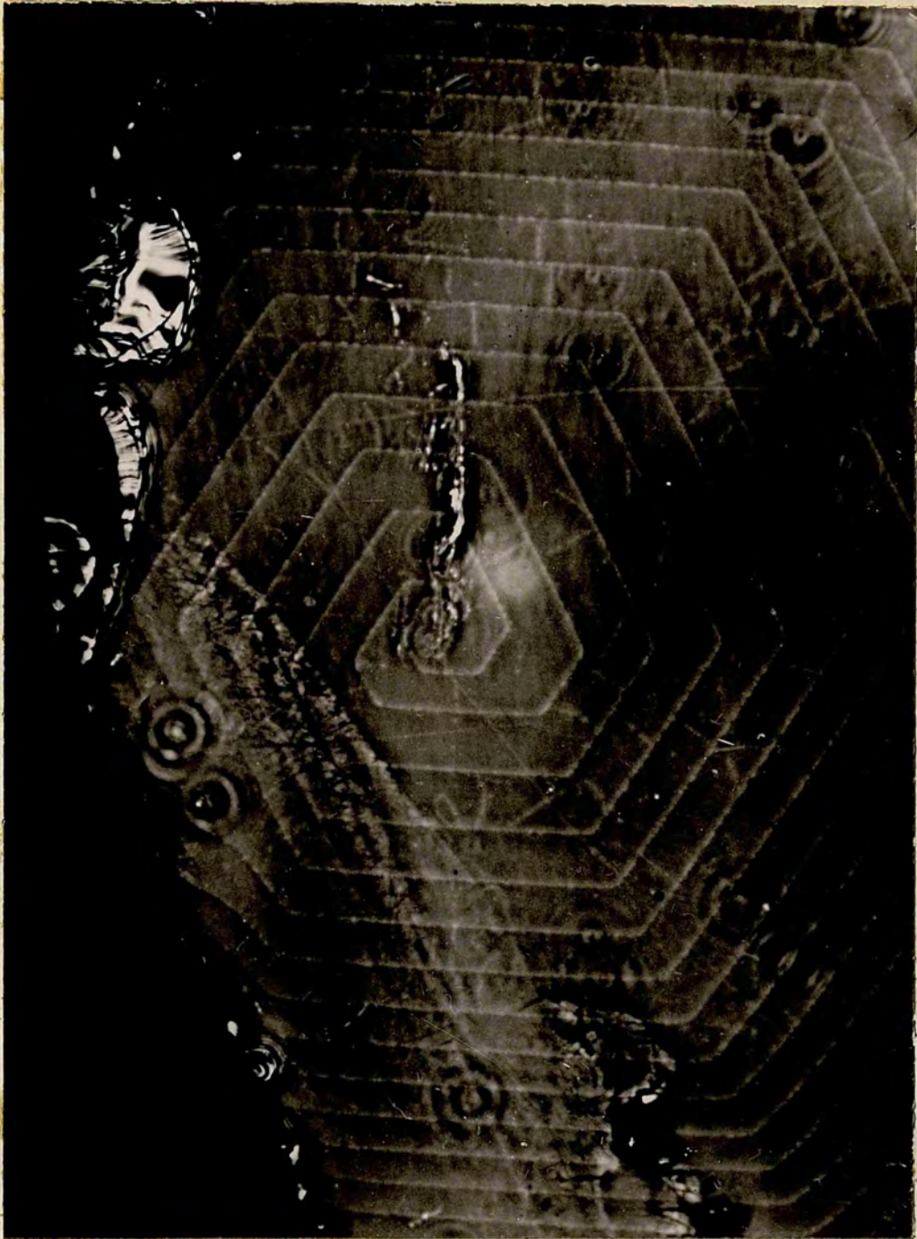
Fig 34. A pair of 'alternately spaced' hexagonal spirals with the central turns rounded observed on a crystal of type 15 R.
