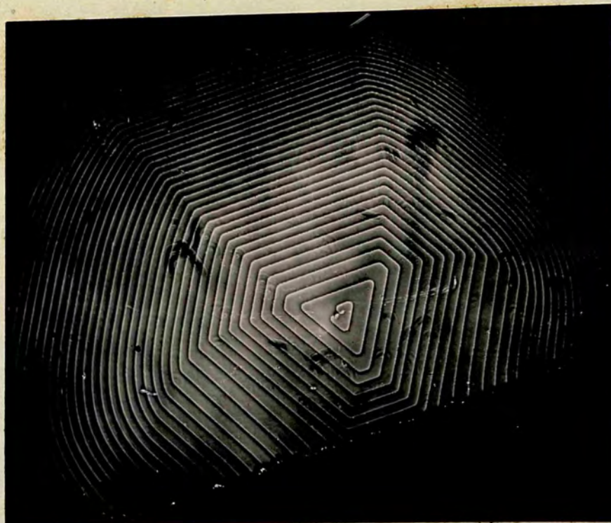
Fig 40. Closed triangular and hexagonal loops from a pair of unlike dislocations.
