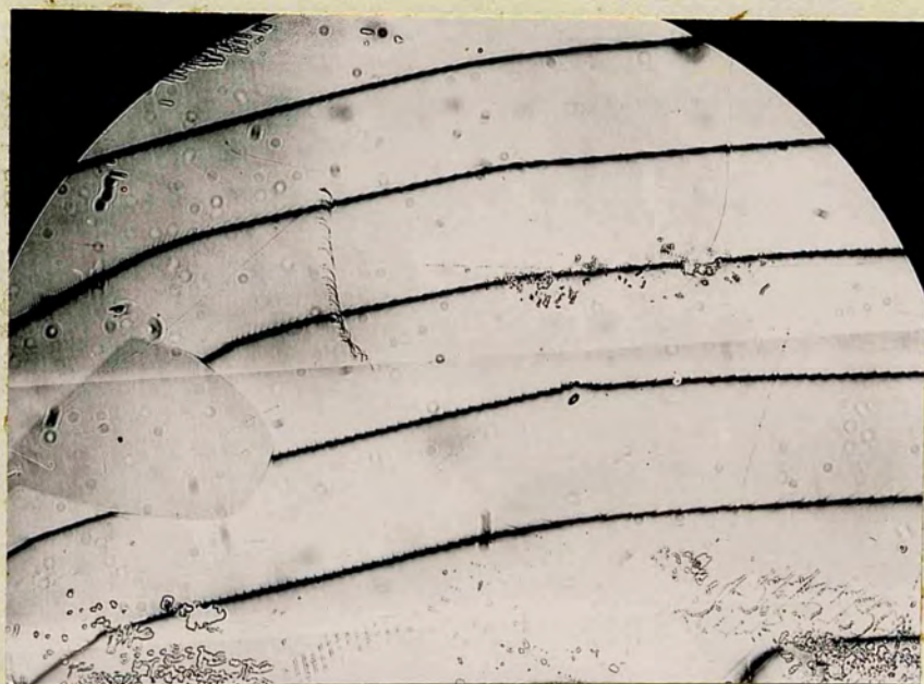
Fig 102. Fizeau fringes passing over the spiral steps of fig 101. Fourth fringe from the top passes over the centre of the spiral.
