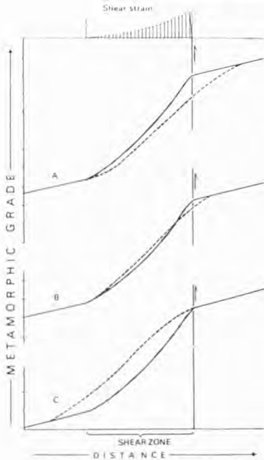
FIG. 7. Graphs showing changes in relative metamorphic grade across a model shear zone at different erosion levels. A, B, C = erosion levels in Fig. 6. Solid curve = grade on displacement. Dashed curve = grade after relaxation.
