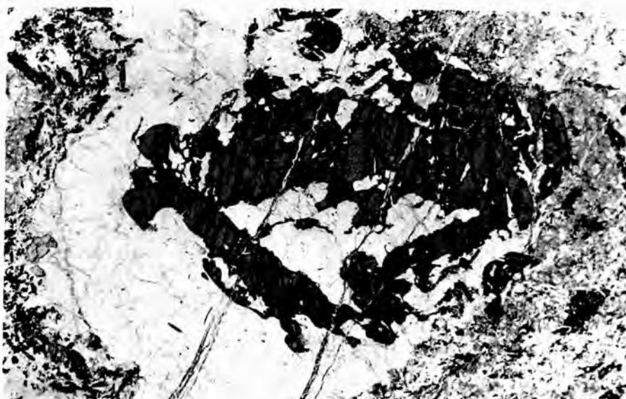
A relict garnet porphyroblast now overgrown by feldspar. Note that the garnet is fractured with numerous fracture planes prior to the feldspar growth. This fracturing is interpreted as a cataclastic texture resulting from very high strain rates. Note too the later inclined fractures which cut the feldspar.
