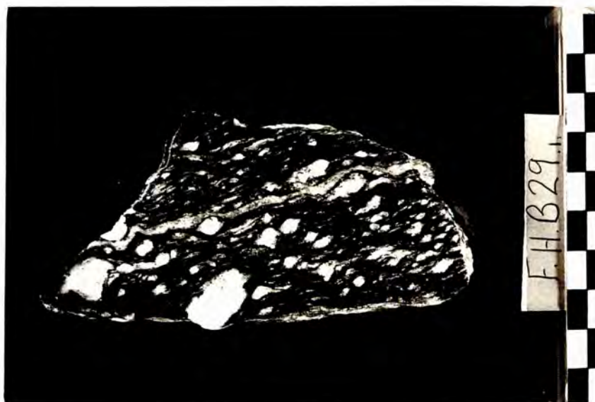
Least deformed specimen in a sequence (Pl.42-45) of mylonitized augen gneiss showing reduction in porphyroclast size with increasing deformation.
