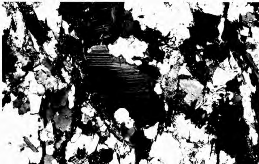
Undulose extinction in a plagioclase crystal. Note the slight bending of the twin lamellae.
