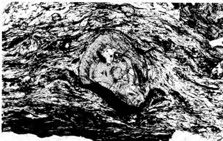
A zoned garnet containing inclusions of quartz and graphite. A large distorted knot of graphite shows where pressure solution (of matrix) has occurred as the schistosity was flattened round the garnet.
