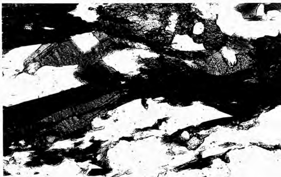
In the bottom of the plate relict biotite crystals are seen overgrown by the leucocratic minerals; this area forms the margin of a small "tectonic pip." The top portion of the plate shows later recrystallised biotites which overgrow the leucocratic matrix.
