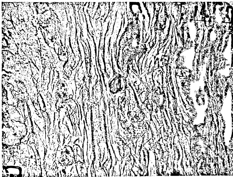
Fig. 4. Salted sheepskin in the wool after storage for 8 months. (X 86).
