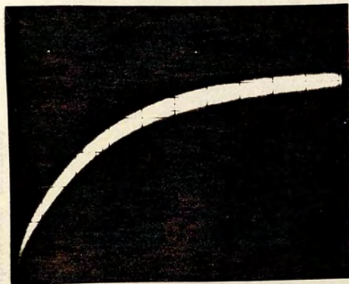
Fig (4-4) Response for steady state overpotential time measurement X-axis = 0.1 ms Y-axis = 20 mV
