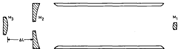
Fig. 1. Optical configuration for generating a single longitudinal mode (not to scale).
