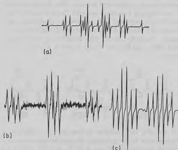
FIGURE 1 The e.s.r. spectra obtained from alkaline solutions of ethylhydroquinone: (a) primary radical in 50% ethanol, 1% NaOH; (b) secondary radical A in 50% ethanol, 10% NaOH; (c) secondary radical B in 10% NaOH
