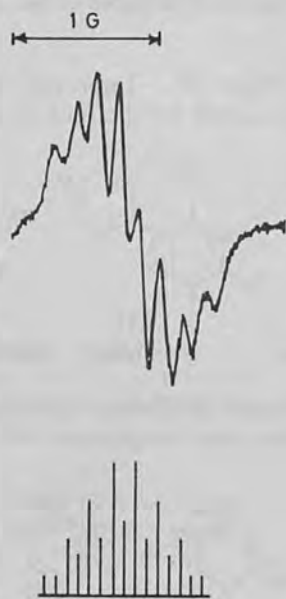
FIGURE 2 One of the side bands of the e.s.r. spectrum of p -nitrophenylsemiquinone, with the reconstructed 'stick' spectrum (alternate lines are 'missing')
