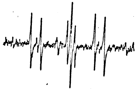
Spectrum of the vinyl-type radicals generated from \cdot\text{CH}_2\text{OH} and \text{HO}_2\text{C}-\text{C}\equiv\text{C}-\text{CO}_2\text{H} ( 1.0 \text{ g l}^{-1} )
